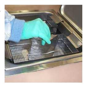
Regular foil testing of your ultrasonic cleaner helps to identify any mechanical problems that may arise.
